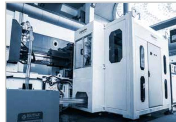
**XTS Series Side Takeout with Mold Stack and Labeling**
